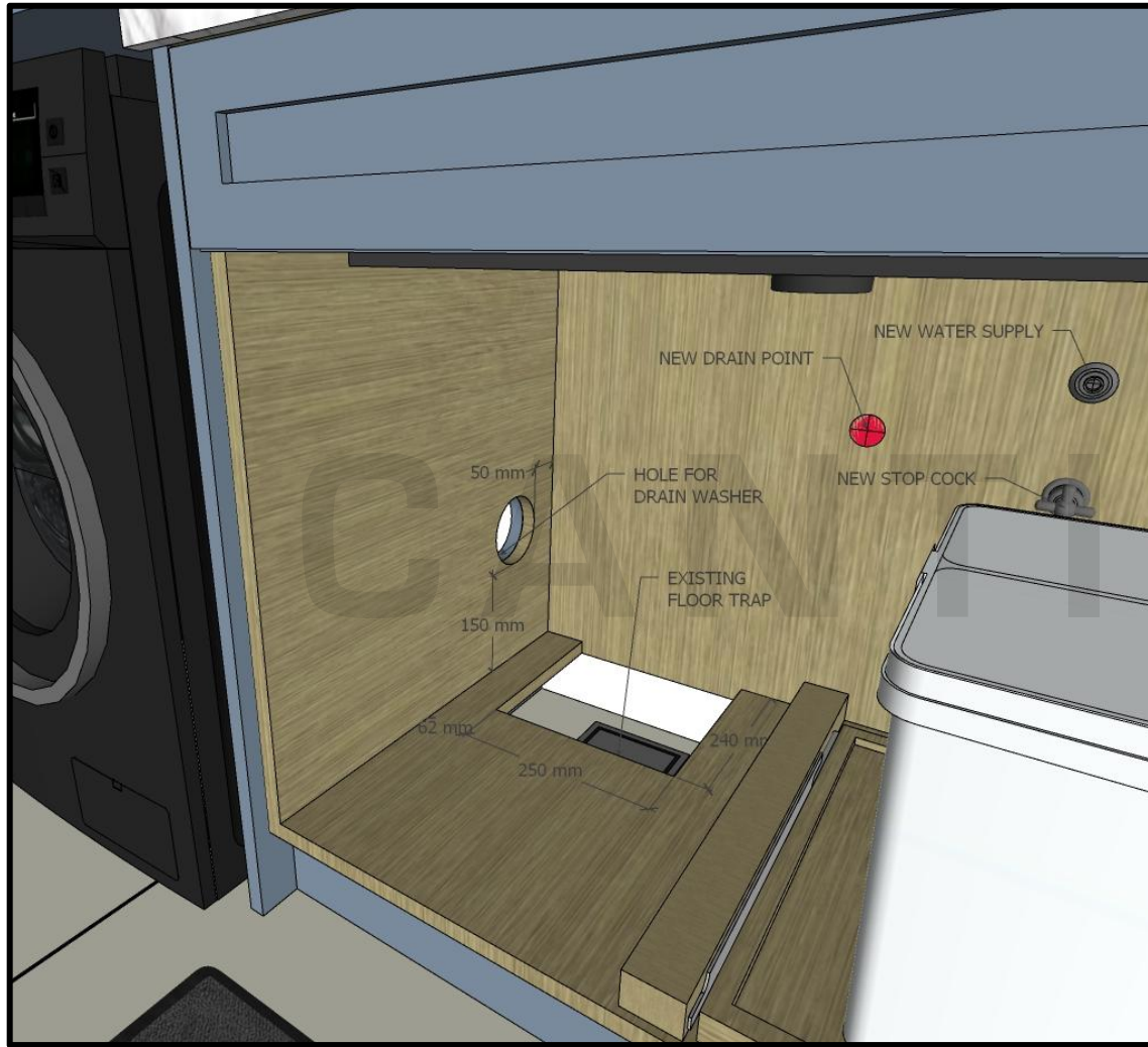
DETAIL A UNDER SINK CABINET
